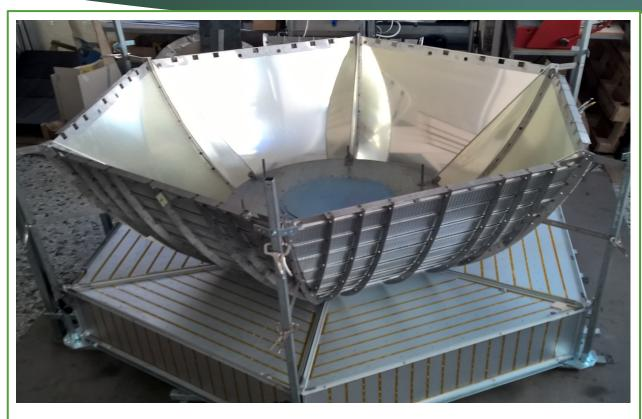
A photo of a partly assembled  $PH_2OS$  Photovoltaic System. The segmented Catenary Solar Collector above, and below the segmented Proto-Traps. This  $PH_2OS$  System offers 4 times the efficiency of system installed in open fields and uses only  $1/4^{th}$  of the surface, and without upwards thermal drafts. Below, is a staging space saving with a  $PH_2OS$  System.
